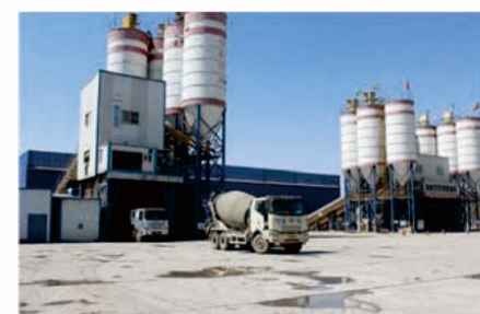
Commercial concrete mixing station
